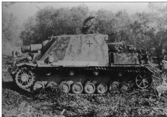
The massive construction of some buildings encountered during the street fighting in Stalingrad induced a demand for a heavy assault gun. The result was the Brumbär (Grizzly Bear), based on the PzKpfw chassis, which mounted a 150mm L/12 howitzer in a fixed superstructure. (US National Archives)
