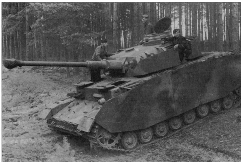
The Ausf. H had 80mm integral front armour and was fitted with side skirts and a turret girdle of spaced armour to protect it against hollow charge ammunition. The colour scheme of this particular vehicle, serving with a Waffen-SS division, is basic German dark yellow oversprayed with large dark green and rust-red patches. (Bundesarchiv)
